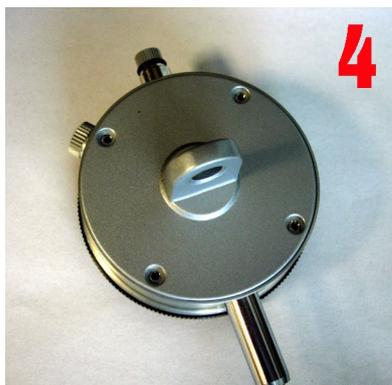
4. Replace the back of the dial gauge in the position shown and replace the screws.
